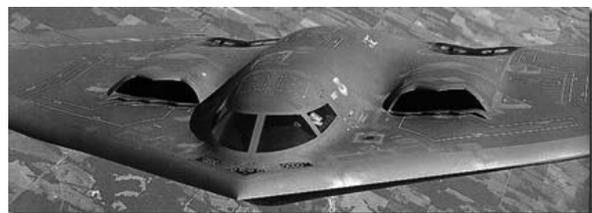
The B-2 bomber, a radar evading long range bomber developed by Northrop Grumman that first saw combat in the 1999 air war over Kosovo.
